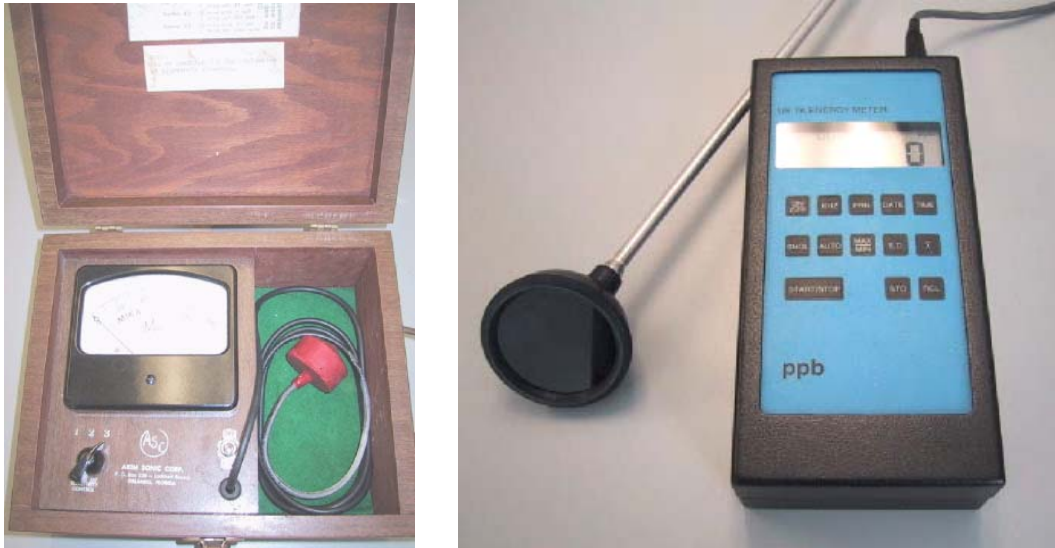
Illustration 6 – Two “probe” type instruments. The one on the left is circa 1958 while the one on the right represents the latest technology (courtesy of ppb, 740 13 th St., Ste. 326, San Diego, CA 92101). Devices of this type are suitable for measuring day to day consistency in a given tank or for comparisons of tanks of similar manufacture.
