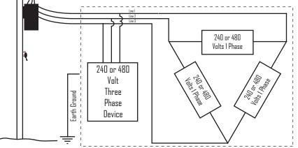
Note - The ground connection is not part of the circuit in the 240 or 480 volt three phase delta supply. It is used as a safety only and is connected directly to the earth ground.
