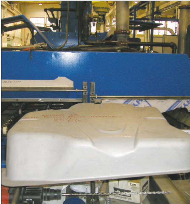
This large chain-conveyor washer is being installed by ICA Cinetic to clean the stamped halves of vehicle fuel tanks (shown foreground and right). Critical in the operation is not only cleaning stamping oil and residue from the parts but also the final drying stage, since water can corrupt the welding process.
